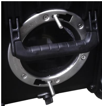
Place Carriage Bolts in Flange
